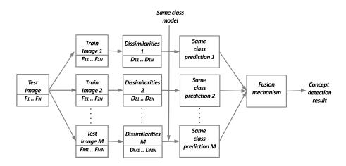
**Fig. 1.** A vector of dissimilarities for the set of used features is computed between the image to be annotated and the each of example the images that belong to the concept. These vectors are fed to the "same class" model and the predictions are fused to obtain a final prediction for the membership of the test image to the particular concept.
