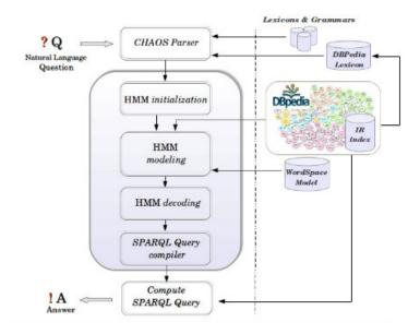
Fig. 1. The overall architecture of the RTV QA system
