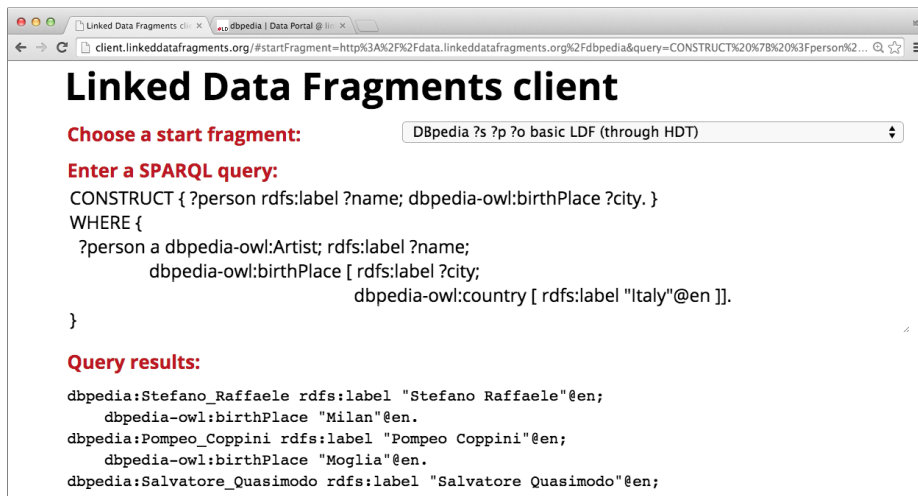
Fig. 1. The demo shows how Linked Data Fragments clients, such as Web browsers, evaluate SPARQL queries over datasets offered as inexpensive triple pattern fragments. In the above example, a user searches for artists born in Italian cities.
