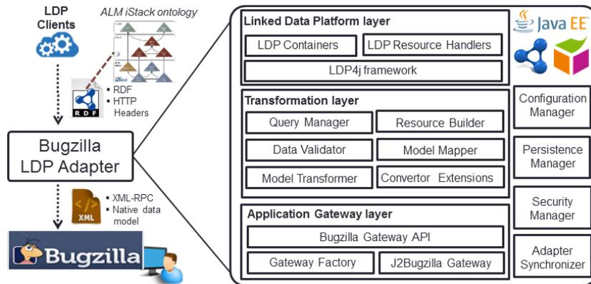
Fig. 1. High-level architecture of the Bugzilla adapter
