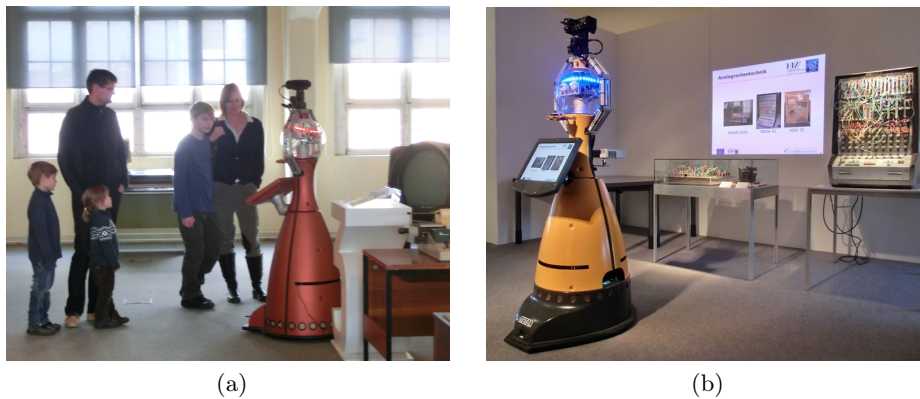
Fig. 2: (a) Tour guide robot leading a group. (b) Attached digital image projector is used to present content.
