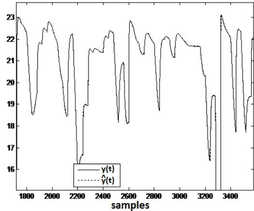
Figure 13. Concentration outputs from reaction tank and NN model for the same set of inputs
