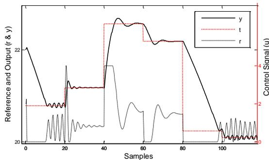
Figure 14. Signals of reference, control and plant output for a MPC structure using a NN model for the control of a chemical reaction tank
