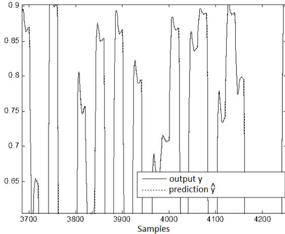
Figure 10. Output of valve and NN model for the same set of inputs
