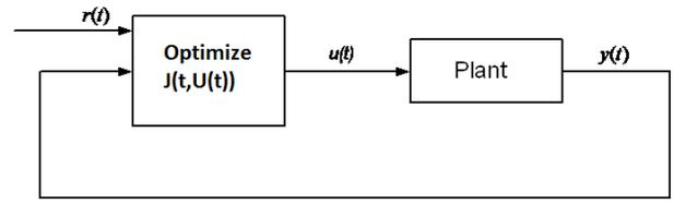
Figure 5. Simplified predictive control structure
