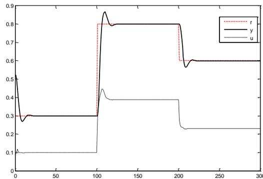
Figure 11. Signals of reference, control and plant output for a MPC controller using a NN model for the control of a valve
