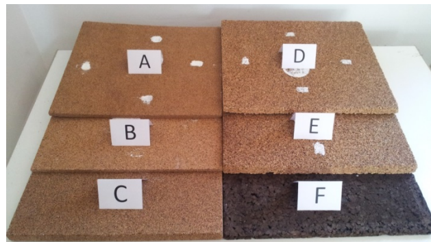
Fig. 1. Testing specimens of agglomerate cork panel.
