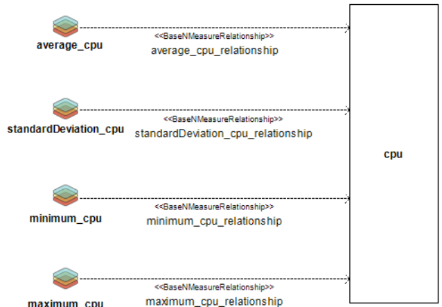
Figure 3: CPU Category Diagram, CPU associated metrics modelled in Modelio SMM
