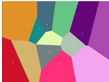
Fig. 2. Voronoi diagram for 13 points (in white). Each element is presented in a different color
