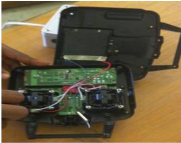
Plate 2. Pigtail antenna on the control board
