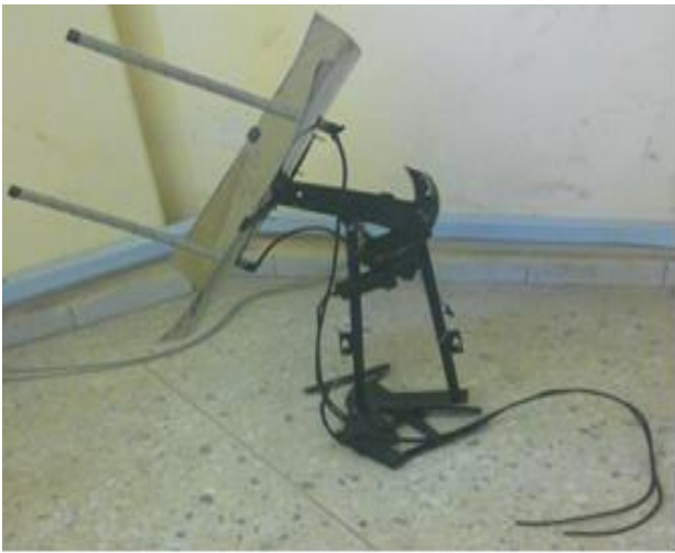
Plate 5. The helical antenna mounted on the Dual axis motorized stand
