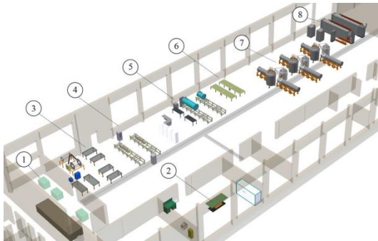
Figure 1. Schematic 3d-view of the facility halls and main equipment placement: 1 – Nuclotron-type SC cable production hall; 2 – magnet winding production hall; 3 – assembling the yoke of the magnet and winding, welding and brazing cooling channels of magnets; 4 – room temperature magnetic measurements; 5 – checking vacuum tightness of cooling channels, beam pipes and cryostats; 6 – assembling magnets in cryostats; 7 – cryogenic tests of magnets at 6 benches; 8 – power converters hall
