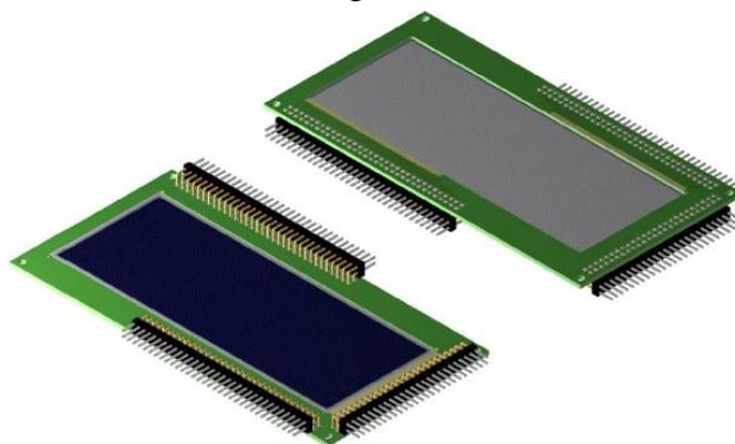
Figure 1a. DSSSD  $48 \times 128$  strips focal plane detector of the Dubna Gas-Filled Recoil Separator spectrometer
