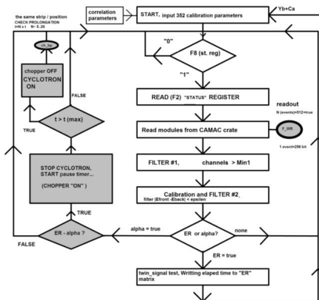
Figure 2b. The flow chart of the ERAS C++ program. Branch for searching for ER-alpha sequences is shown in gray in the left picture side. Calibration parameters are extracted from  $^{nat}\text{Yb} + ^{48}\text{Ca} \rightarrow \text{Th}^*$  nuclear reaction (352 constants)
