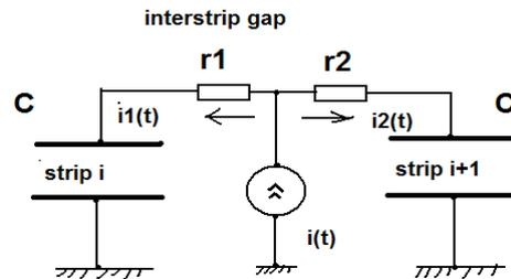
Figure 8. Inter strip charge collection equivalent circuit schematics
