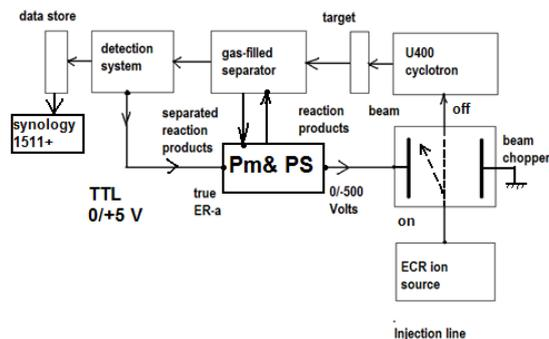
Figure 2a. Block-diagram of the process to search for ER-alpha chains and to provide beam stops. (Pm& PS – parameter monitoring and protection system of the DGFRS)
