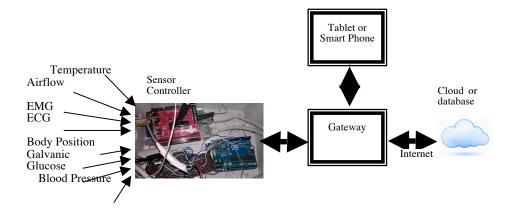
Fig. 1. The architecture of the health monitoring system
