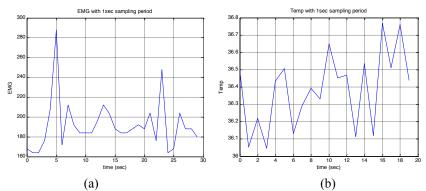
Fig. 3. EMG sensor output for two strong muscle contractions and three less strong muscle contractions in between (a). Temperature sensor output for a person that has a temperature of  $36.5 \,^{\circ}$ C (b).
