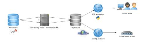
**Fig. 1.** BioKB platform. The publications, initially stored in Solr, are processed by the text-mining module. The results are then stored in Virtuoso for dissemination through a web interface and a SPARQL endpoint.
