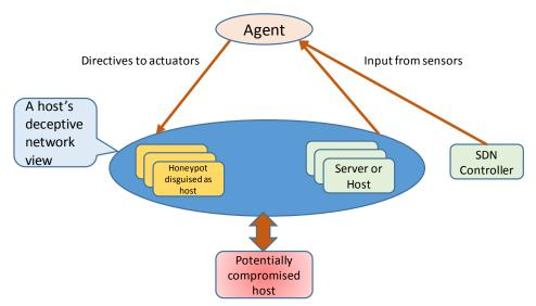
Figure 2. Agent interacting with a potentially compromised host through a deceptive network view
