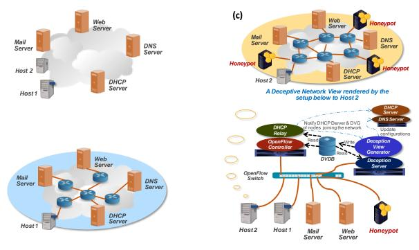
Figure 1. ACyDS enables rendering of different network views to hosts on the same physical network
