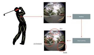
Figure 3. Motion capture with a small omnidirectional camera.
