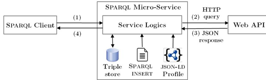
**Figure 2: Example implementation of a SPARQL micro-service.** A JSON-LD profile interprets the Web API JSON response as a temporary graph  $G$  stored in the local RDF triple store. An INSERT query optionally augments  $G$  with RDF triples that JSON-LD cannot yield. Lastly, the client’s query is evaluated against  $G$ .
