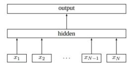
**Figure 3.** Model architecture of FastText for a sentence with N ngram features  $x_1, \ldots, x_N$ . The features are embedded and averaged to form the hidden variable
