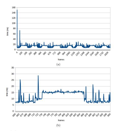
Fig. 2: (2a) describes the time occurring for the feature extraction frame by frame. (2b) shows a zoomed overview on several frames that correspond to a single person passing under the camera.
