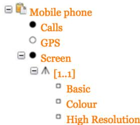
Figure 2: A feature model example (constraints not shown).
