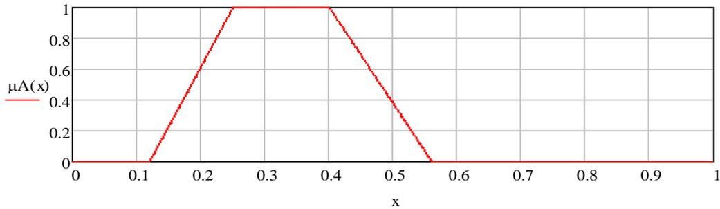
**Figure 2.** The graph of the assignment function  $\mu_A(x)$  for the intensity (mm per minute) of the average “autumn” rain  $I_{\min} = 0.12$ ,  $I_0 = 0.25$ ,  $I_1 = 0.40$ ,  $I_{\max} = 0.56$ .
