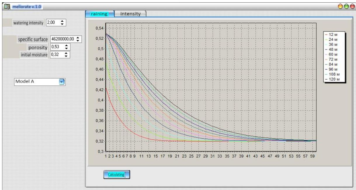
**Figure 5.** Operation of the software for calculating humidification profiles for sprinkling and drip irrigation.
