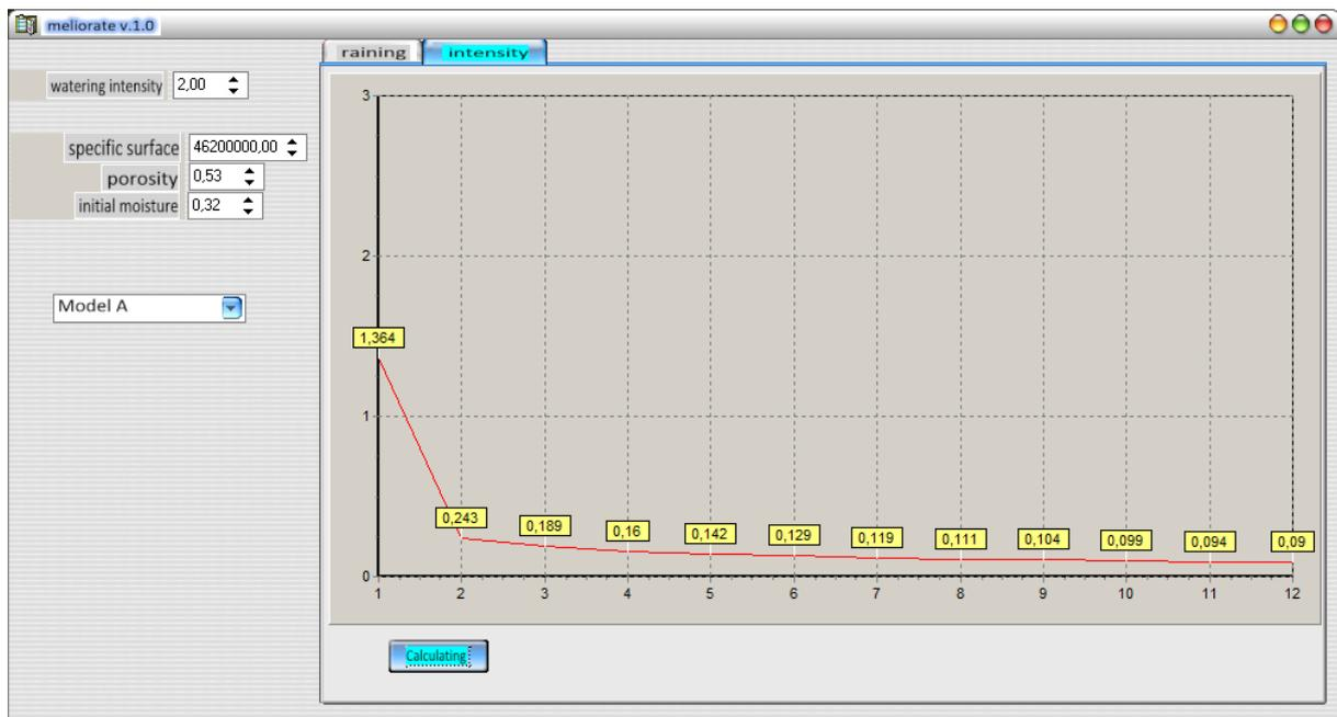
**Figure 4.** Work of the software for calculating the absorption rate.
