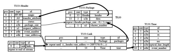
Figure 2. Auto-generated diagram for TUNKA-133 file format specification presented in KAITAI STRUCT
