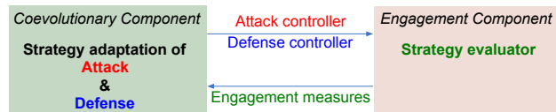
Figure 1: Component overview of our coevolutionary adversarial AI framework. The coevolutionary component performs search over the adversary controllers. The engagement component evaluates the strategies of the adversaries and returns the measurements of the engagement.
