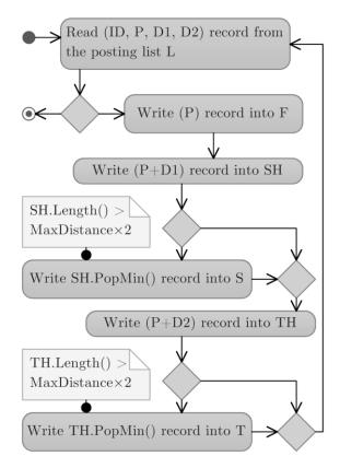
Figure 5 UML diagram of the posting list reading process.
