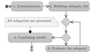
Figure 2 UML diagram of the search algorithm general structure.
