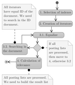
Figure 3 UML diagram of a subquery evaluation.
