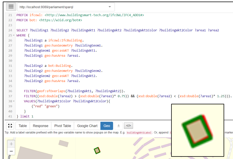
Fig. 3. SPARQL to align overlapping building geometries. Screenshot is taken from YASGUI, the Geo results page draws the ifcOWL (red) and BOT (green) geometries.
