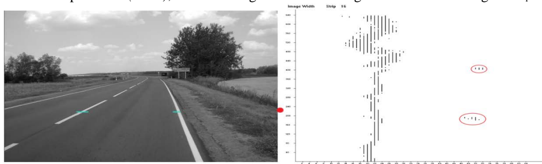
Figure 1. A road scene and the geometrized histogram of the grayscale component of the i -th horizontal strip.
