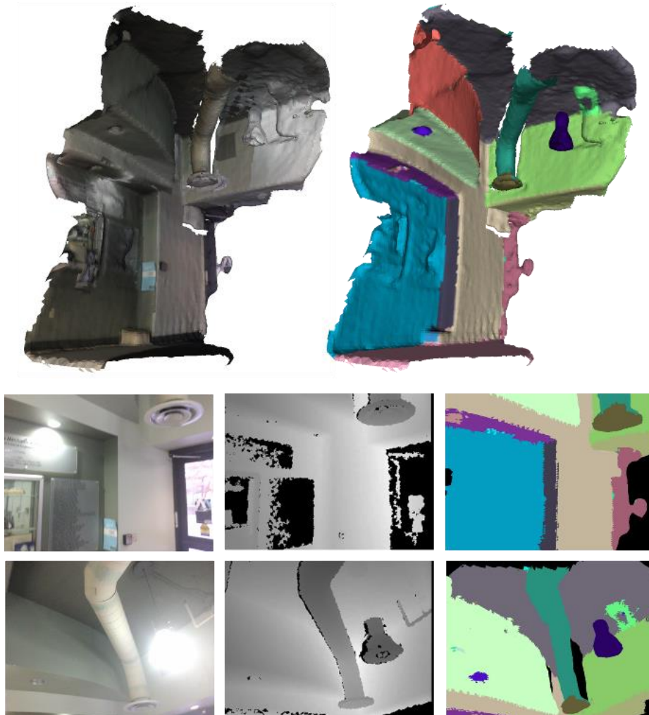
Figure 1: Example of data provided in the 3DFacilities dataset; 3D reconstruction with color texture (scan); 3D reconstruction annotated with instance-level category labels (scan); 2D image color (frame); 2D image depth (frame); 2D image annotated with instance-level category labels (frame)
