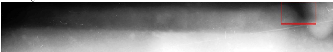
Figure 19. Image No. 2 of the radiographic image with the recognized defect “lack of fusion”.
