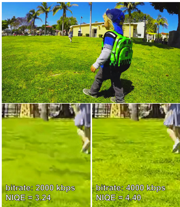
Fig. 11. Frame 58 from Playground video sequence, codec: x265, ripping use case. According to NIQE, left image is visually better.
