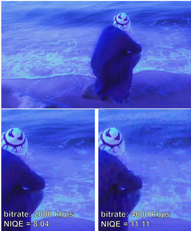
Fig. 3. Frame 208 from Hera video sequence, codec: x264, fast use case. According to NIQE, left image is visually better.
