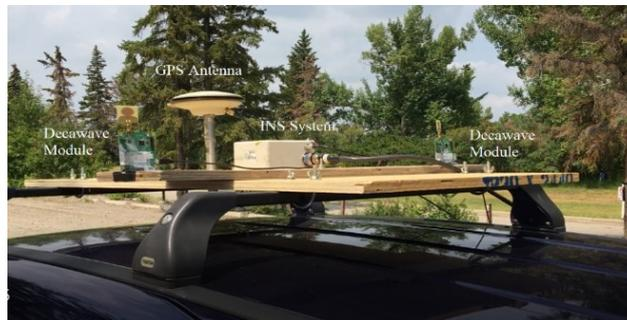
**Fig. 3.** Installation of two UWB modules, GPS and INS on a moving vehicle.
