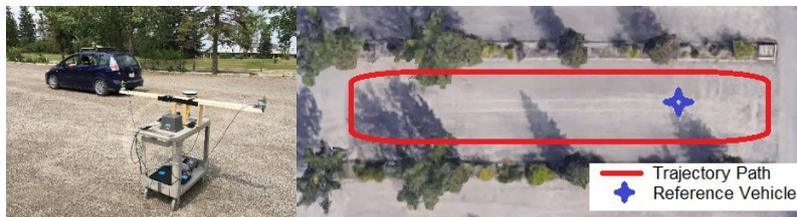
**Fig. 4. :** Field test scenario showing (a) the vehicles used and (b) the trajectory of the moving vehicle.
