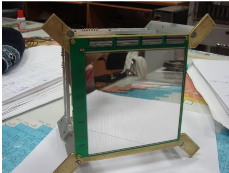
Figure 4. Focal detector 128 \times 128 strips
