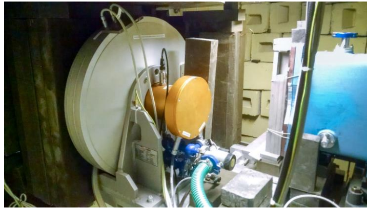
Figure 1. The new Fourier chopper on the HRFD spectrometer
