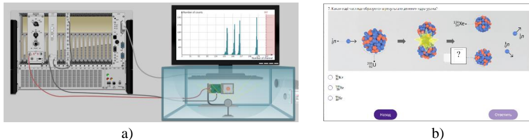
Figure 5. a) Virtual Practicum on Nuclear Physics. Investigation of the interaction of charged particles with matter. Semiconductor detectors for alpha-particle registration b) Final Quiz
