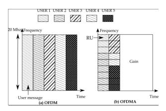
Fig. 2. Configuration of RUs on a 20 MHz band
