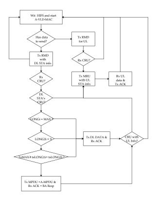
Fig. 4. Flowchart of the transitions of A-VLD-MAC.
