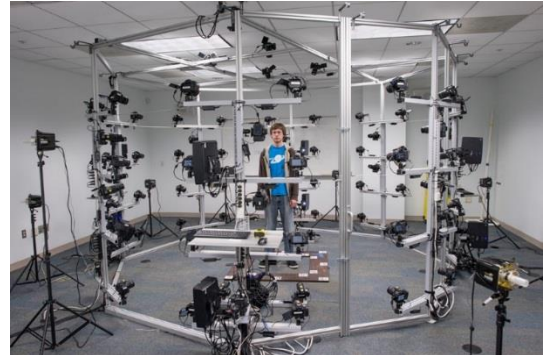
Fig. 1. Example of Studio, which allows getting a set of images from different angles [4].
