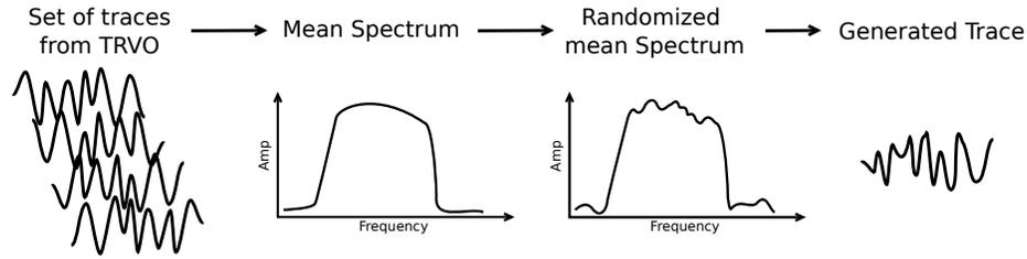
**Fig. 2.** Schematic representation of noise generation from the TRVO data.
