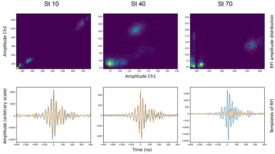
**Fig. 1.** Top: channel-to-channel RMS distributions of the found RFI. the red circle is the distribution core. Bottom: templates of RFI.
