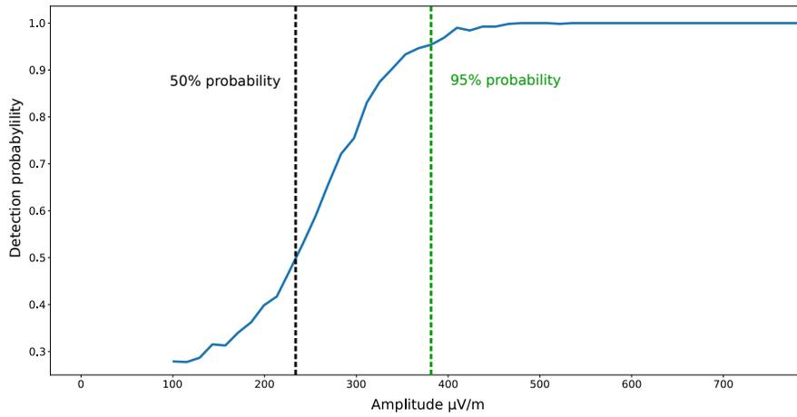
**Fig. 4.** Dependence of detection probability on signal amplitude.
