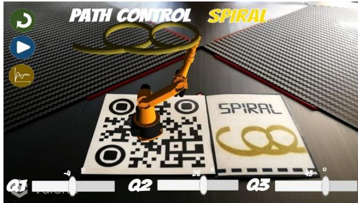
Fig. 19. Robot arm movement on the spiral path when applying control.
