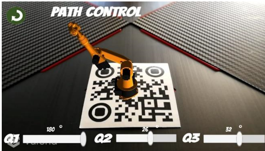
Fig. 14. Manual control of the robot arm when changing parameters q_1 , q_2 and q_3 .
