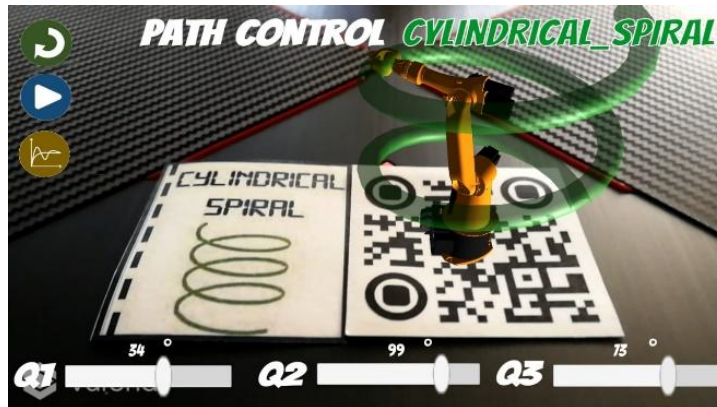
Fig. 22. Motion of the robot arm on the cylindrical spiral path when applying control.
