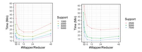
**Fig. 5.** Runtime of SEPP on the MSNBC dataset with different minimum support thresholds, in relation to different numbers of mapper/reducers.
