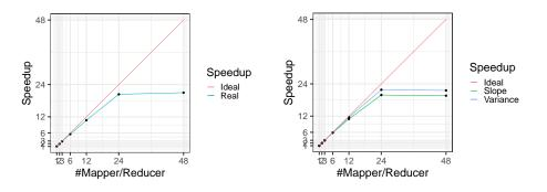
Fig. 3. Speedup of SEPP (support quality function) on 27M, in relation of the applied number of Mappers and Reducers.
