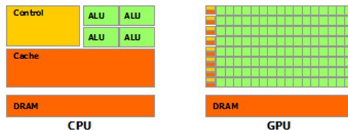
Figure 2: Comparison of CPU and GPU structures
