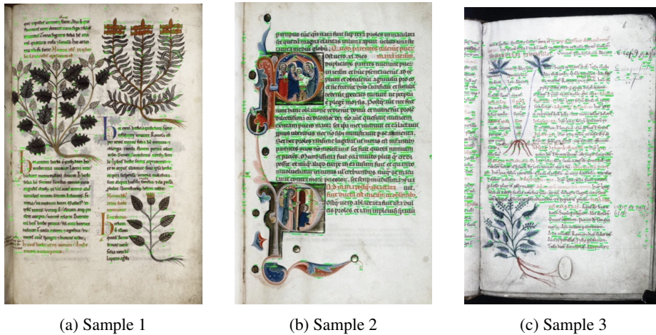
Fig. 4: Text and image extraction for different samples of manuscripts. This shows that the algorithm can handle difficult cases such as: single and double columns of text, text lines which are broken by illustrations inserted within the text column, images including facing pages of the manuscript, and images including extraneous material, such as the space outside of a book.
