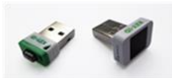
Fig. 1. Hardware keys: with a button (left) and with a fingerprint scanner (right)
