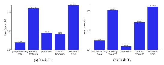
**Figure 3:** Disaggregated total time for both tasks. The time elapsed in each stage of the input processing is shown in base-10 log scale (Y-axis). Time is reported in seconds.
