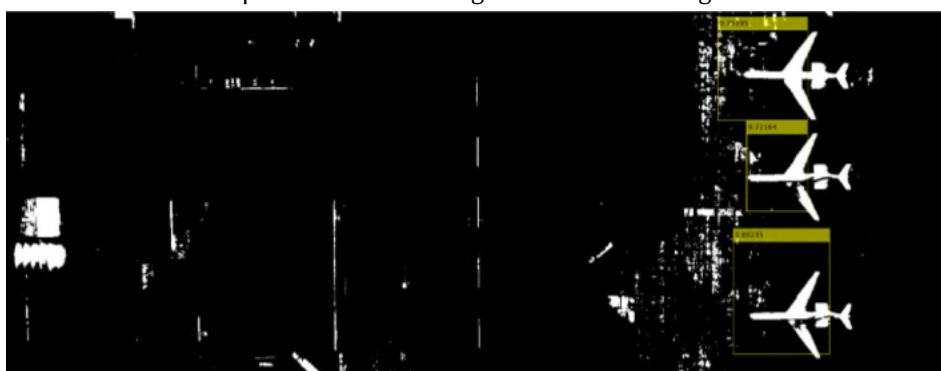
Figure 2: The result of using a feature model of an aircraft for its recognition.
