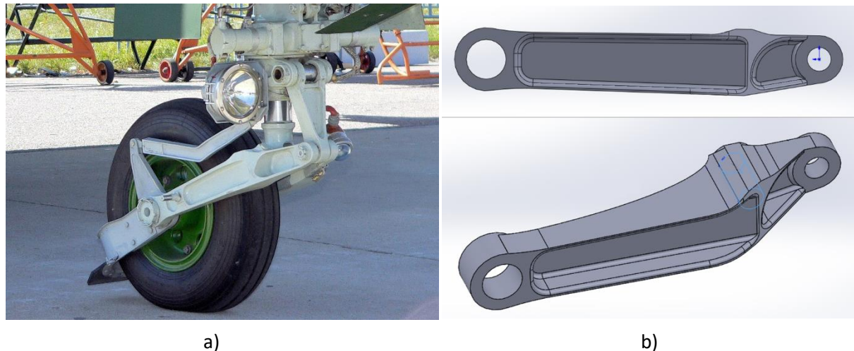
Figure 3: a) photo of the front landing gear of the Yak-130 aircraft, b) 3D model of the fork
