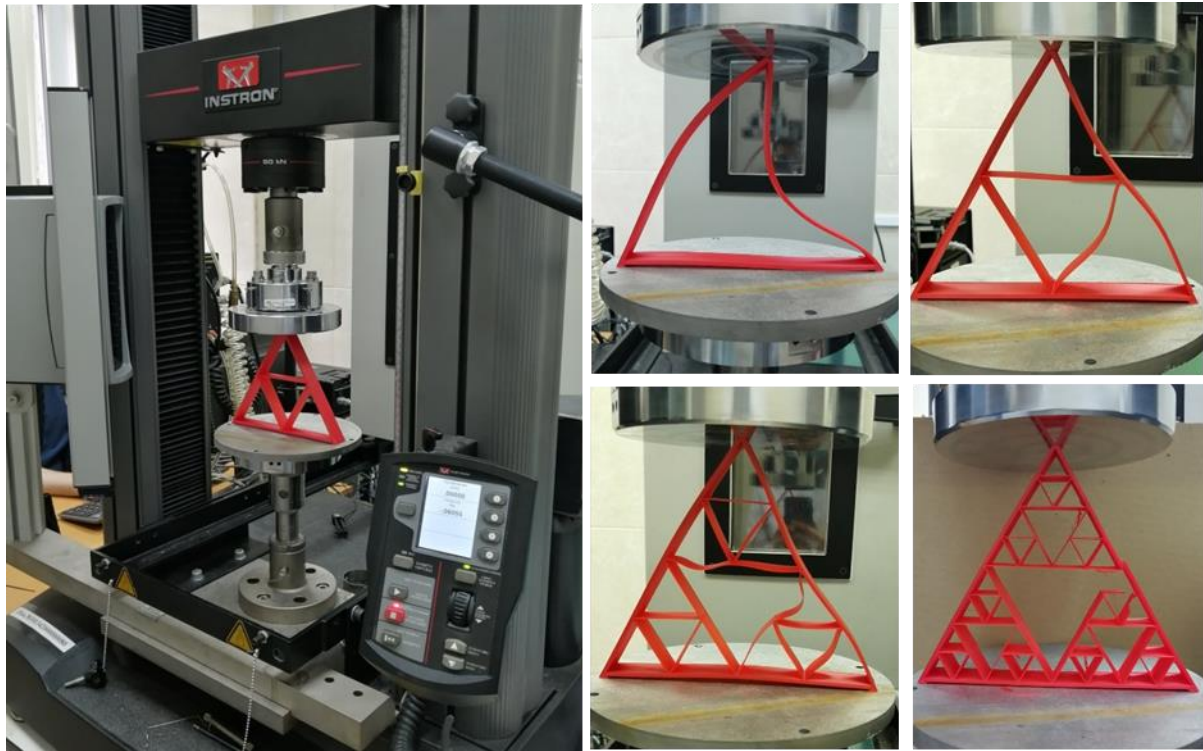
Figure 6: Strength tests of plastic Sierpinski triangle models
