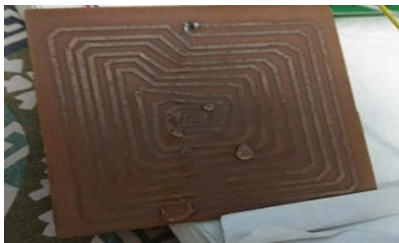
Figure 4: Wet sensor showing wet condition
