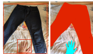
Figure 7: Bounding box approach (left) compared with the Pixel approach (right). This is an example misclassification by the Bounding Box approach (the rectangles are contained one into the other) and correct classification by the Pixel based approach (the pixel masks have no pixel in common).
