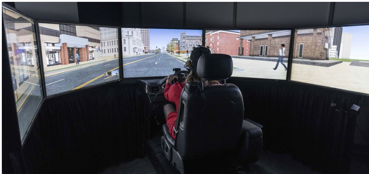
Figure 1: A high-presence driving simulator can be used to provide a training experience, or can be used to test the effects of experiential training.
