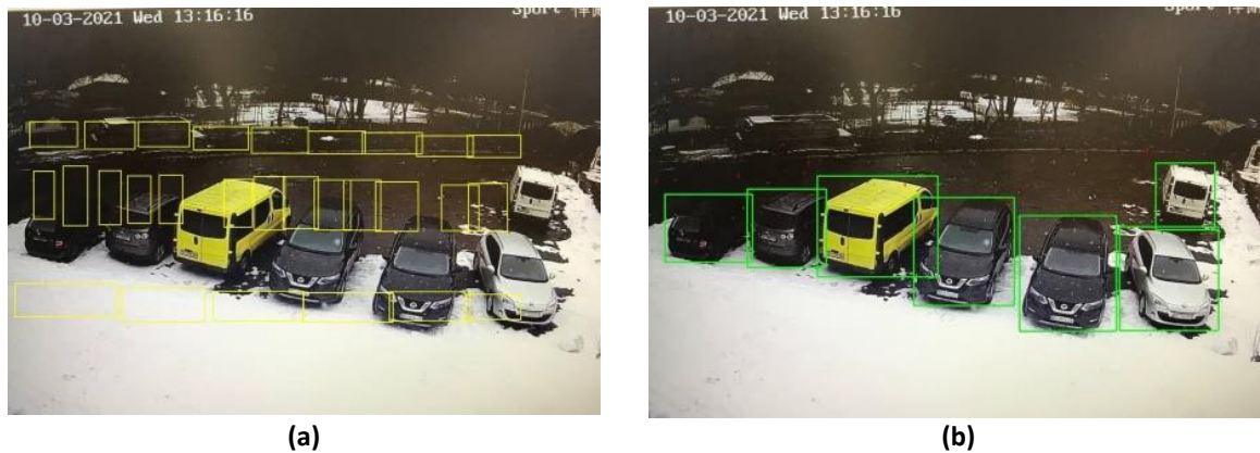
Figure 3: Identified objects on the target image that correspond to the searched cars, found by: (a) – OpenCV + CNN, (b) – GCV API [23]
