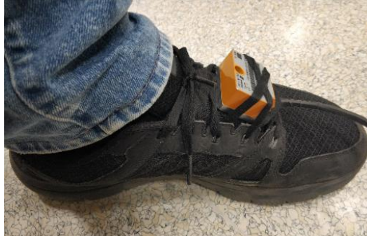
Figure 3: STIM300 attached to the foot via shoe's laces.
