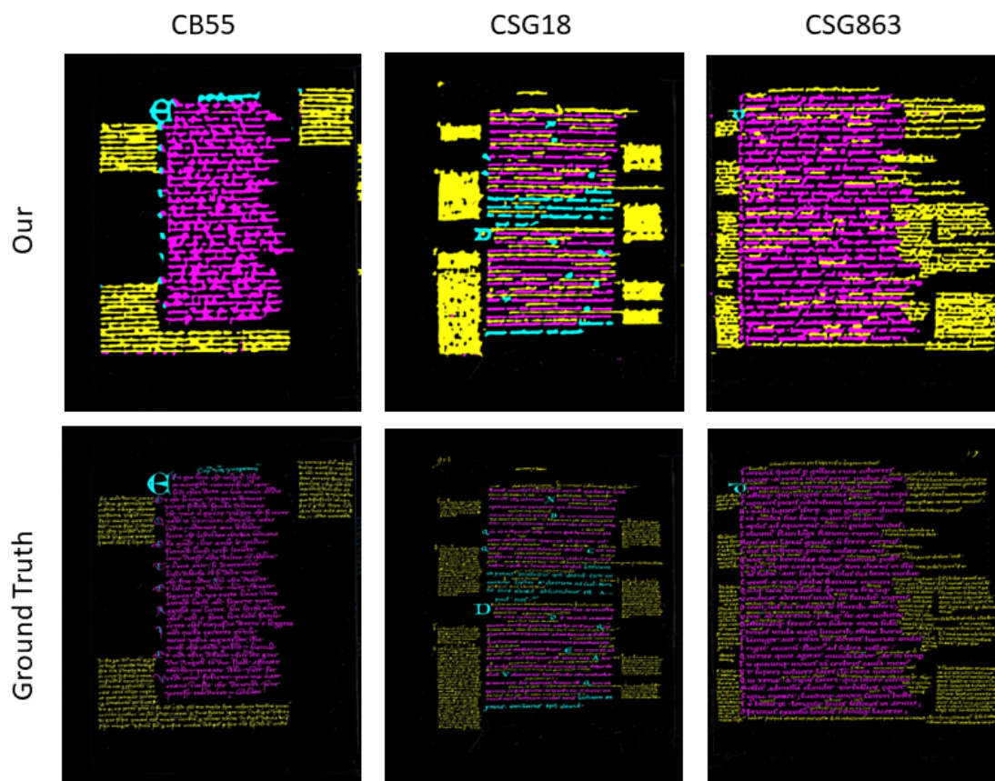
Figure 5: Image shows the comparison between the segmentation results obtained by our framework and the ground truth provided by DIVA-HisDB. Each column represents a different instance of the three classes of manuscripts.
